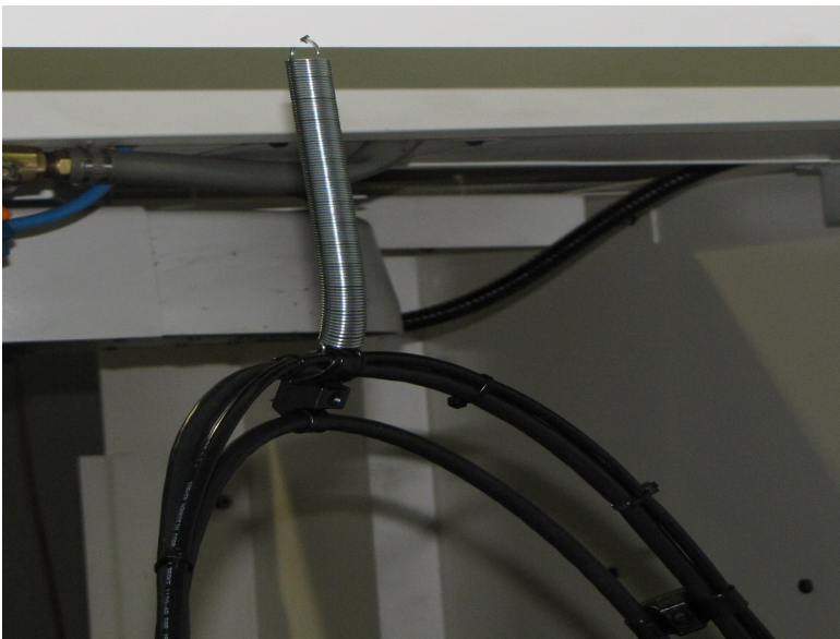
Figure 9, Spring to hold cables slack up off the table
