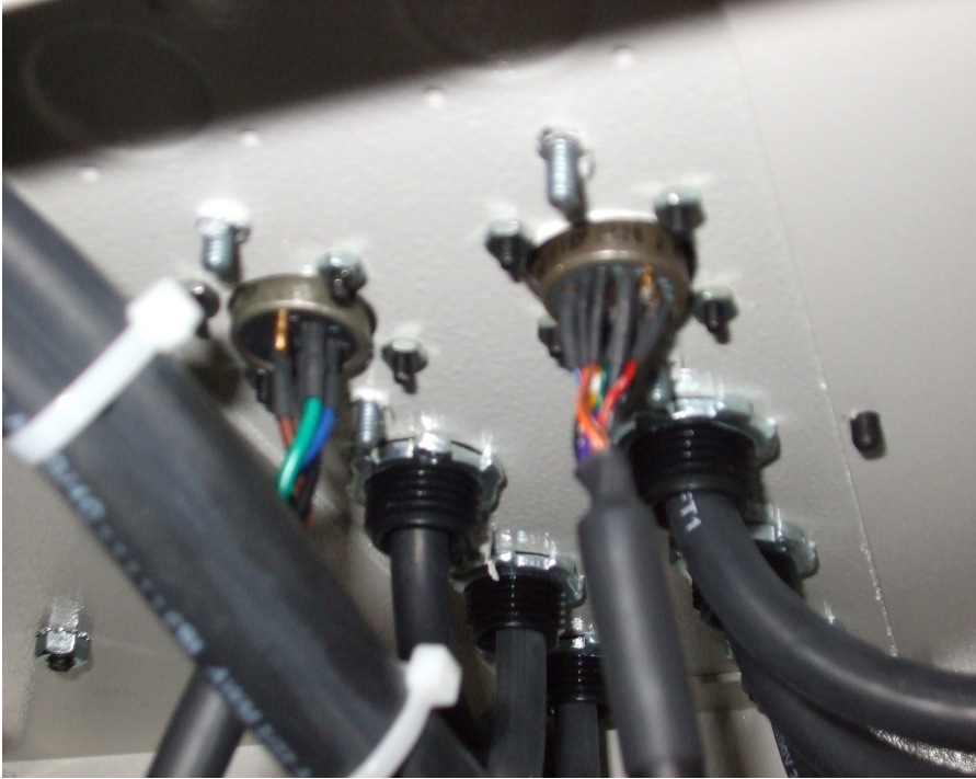
Figure 7. There are two ways to mount the bulk head connectors for the signal and power wires, either inside the work area of the machine or on the electrical cabinet outside the work area. If the electrical cabinet already has knock outs, use those holes. Otherwise, for the power bulkhead you will need a 1-3/4" punch, and for the Signal a 1-1/4" punch to allow the cables to enter the cabinet. The panel mount disconnects can be put either into the work area or on the rear electrical cabinet.
